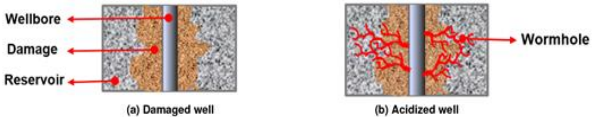
Figure 11. Illustration of matrix acidizing impact on the well (Dong et al., 2020).
