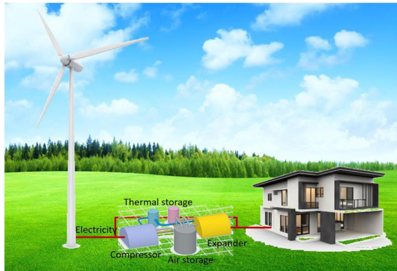
Figure 7. The wind-CAES hybrid system layout (Zhang et al., 2021).
